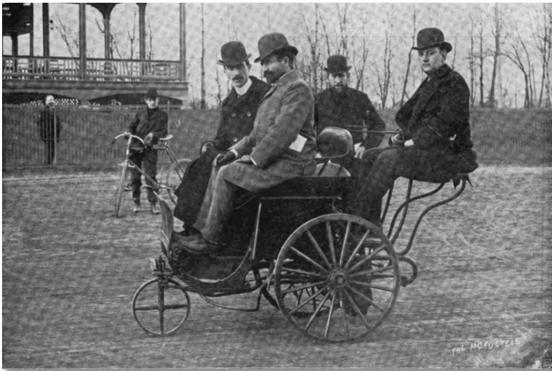
Figure 42. The three-wheeled electric vehicle developed by The Columbia Perambulator Company, which was envisioned as a means to move guests about the 1893 World's Fair ( The Motorcycle , November 1895, 34).
