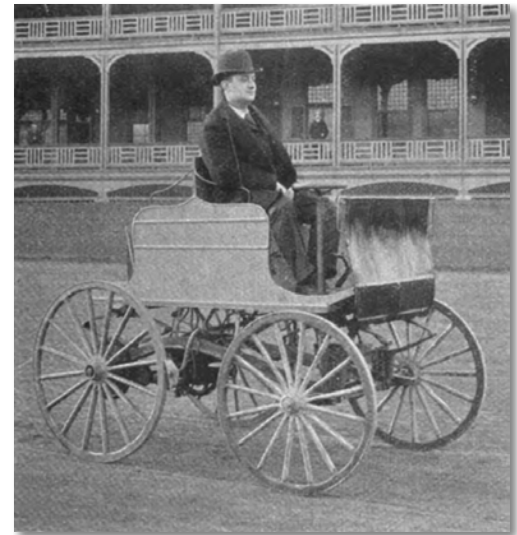
Figure 43. The larger, four-passenger electric vehicle developed by The Columbia Perambulator Company ( The Horseless Age , December 1895, 15).
